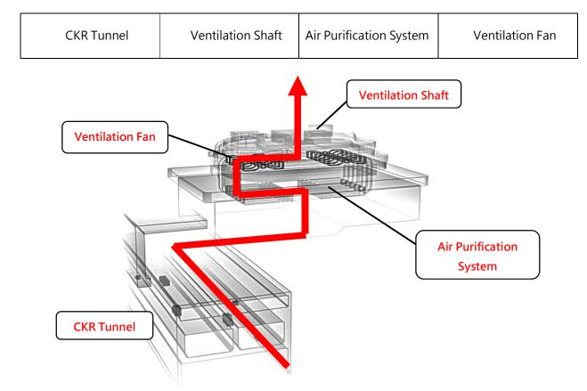
Each ventilation building of the CKR is equipped with three sets of the advanced air purification system and six ventilation fans to discharge purified air to the atmosphere. Please draw the airflow direction on the model above and state the principle.
